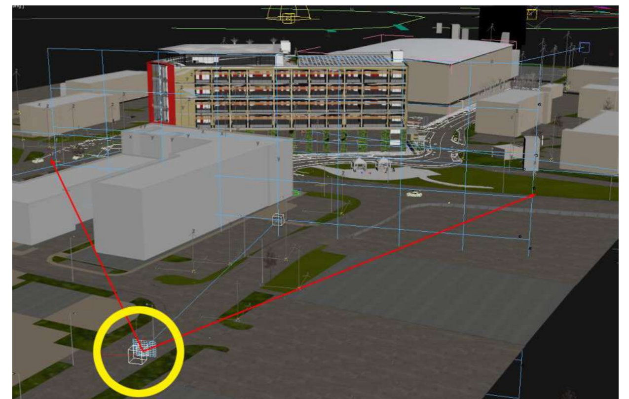
Camera location in model—on survey point
