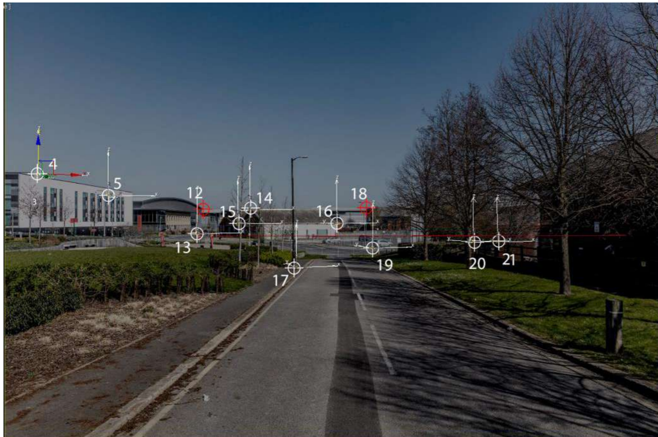
Model viewport shows 3D model survey points aligned to marked up base photo from within the deduced camera
