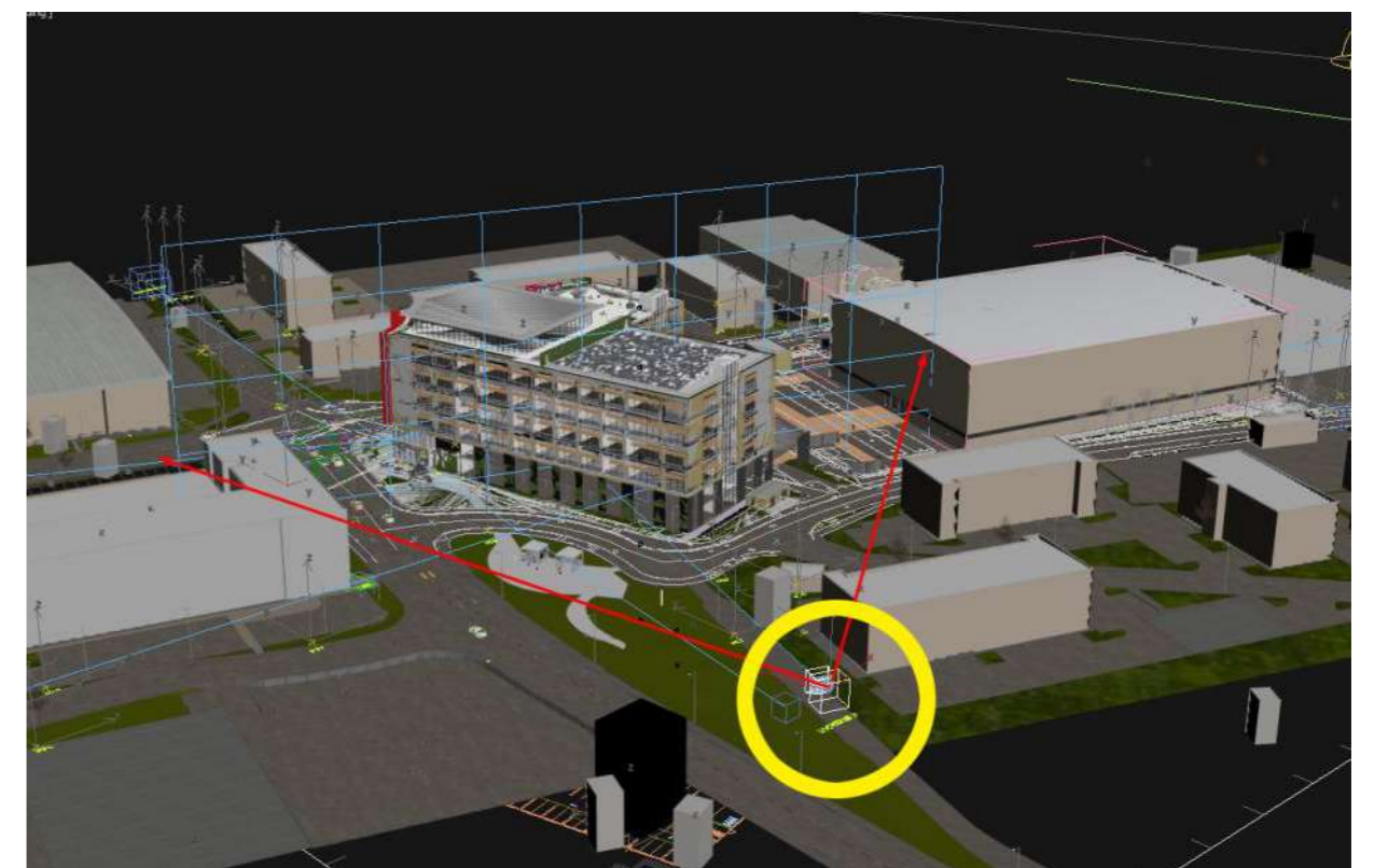
Camera location in model—on survey point
