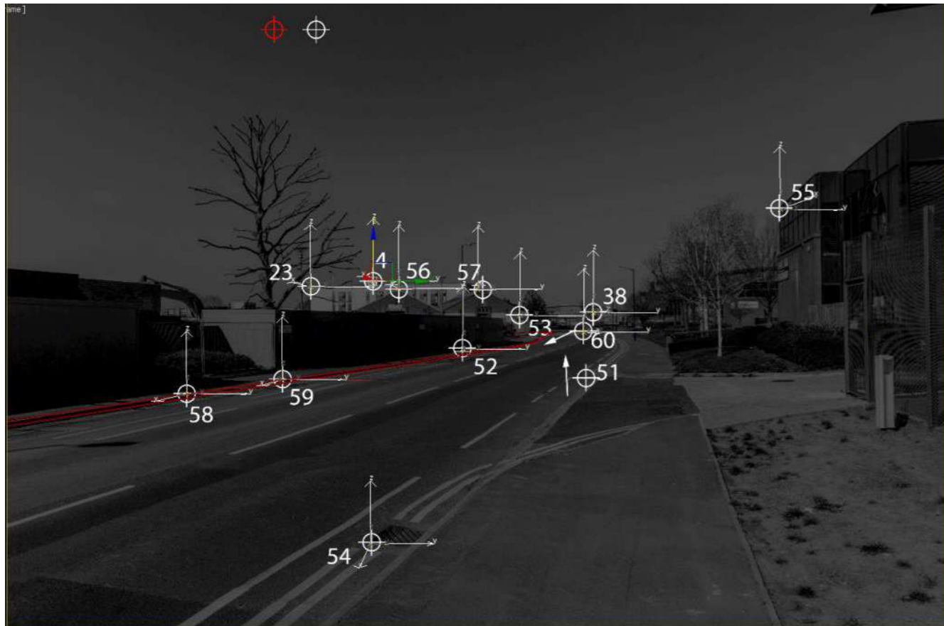
Model viewport showing 3D survey points aligned to marked up base photo from within the deduced camera
